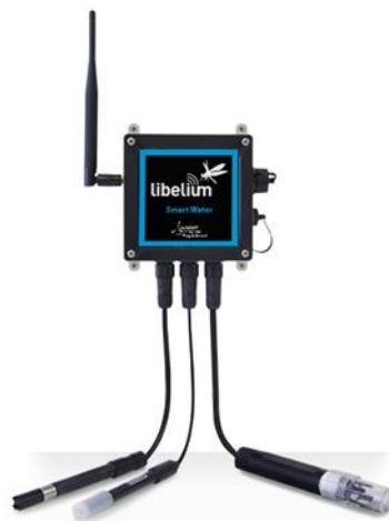
Figura 4. Smart Water Sensor Libelium. 4
